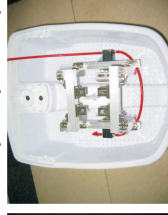
一種多穴, 採用吸抱結合方式取出 Many cavities mold packing by a way of combining absorbing with embracing
