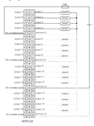
fuse: 10 A max (determined by the module load current), fast blow
