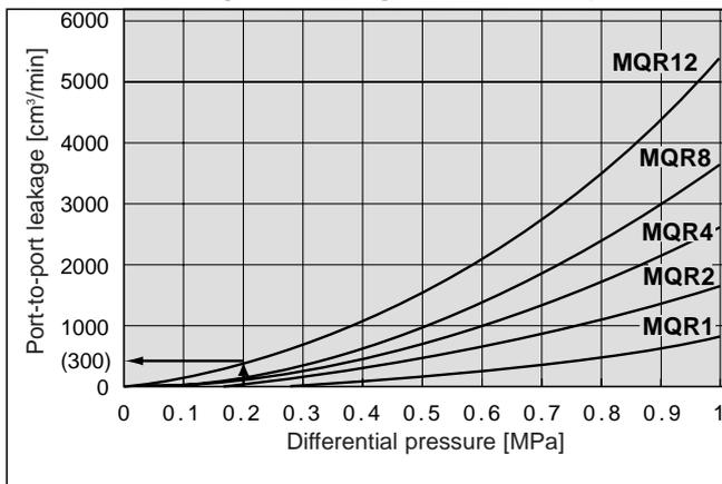
e.g.: If adjacent ports are connected to positive vacuum pressure of -0.1 MPa and 0.1 MPa in MQR12, then differential pressure is 0.2 MPa, and leakage is 300 (cm³/min).
