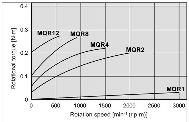
Note 1: Value when no pressure applied. Temperature rise is reduced by supply of air.
