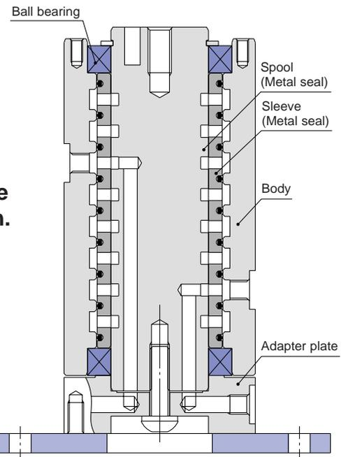
Rotational torque unaffected by supply pressure and temperature fluctuations
