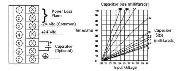
NOTE: A normally closed relay contact rated at 220 Vac, 6A / 30 Vdc, 5A is available on terminals 1 and 2 of the power terminal strip. This contact set may be used to signal input power OFF. The relay will de-energize when input power drops below 8 Vdc.
