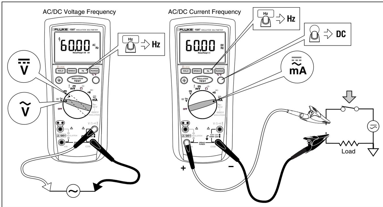
Figure 14. Measuring Frequency
