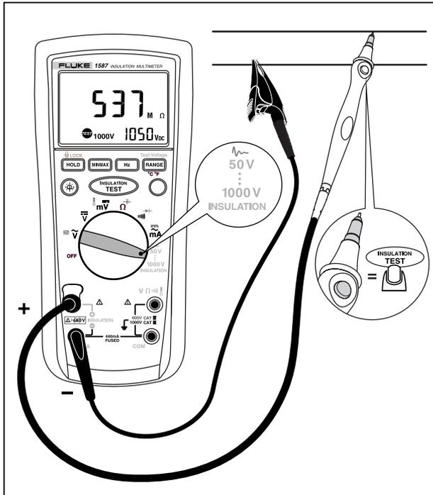
**Figure 13. Testing Insulation**
