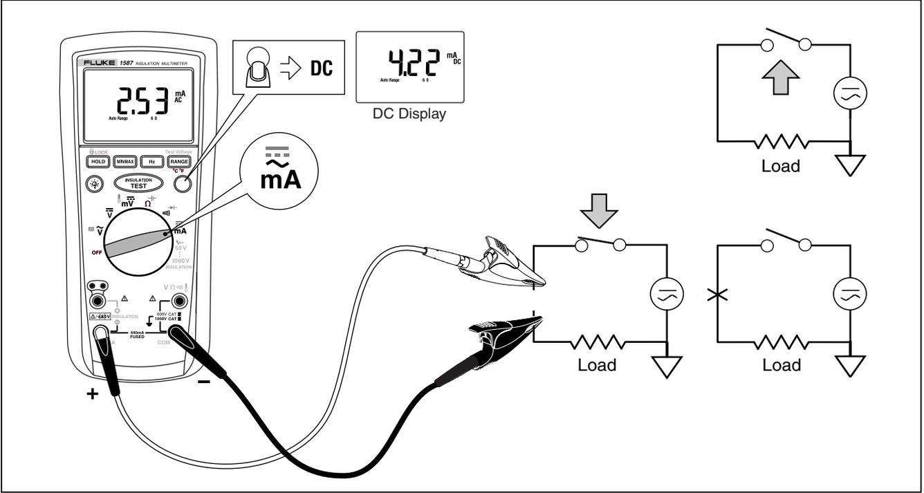
Figure 12. Measuring AC or DC Current
