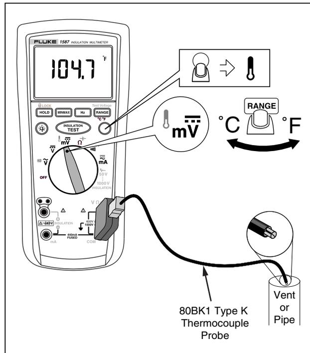
Figure 7. Measuring Temperature
