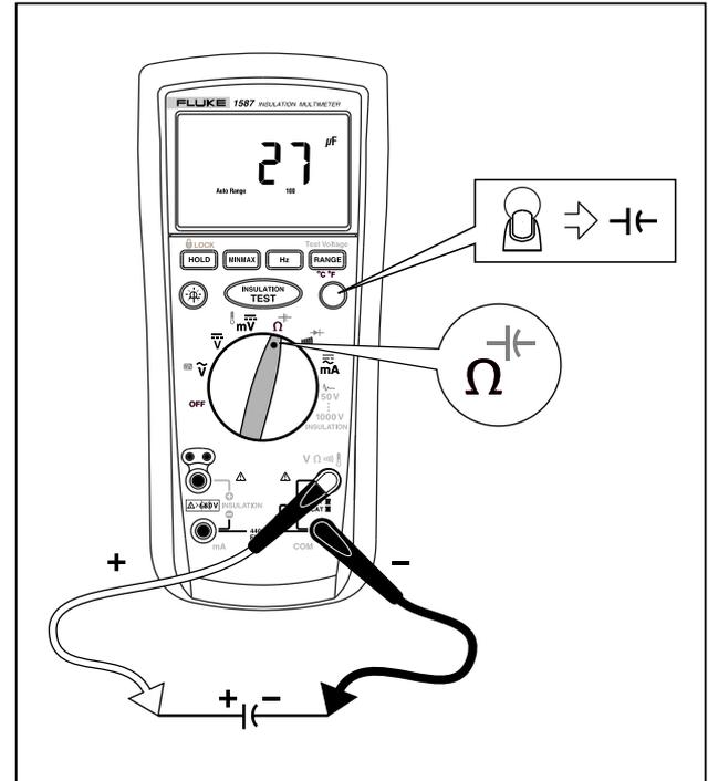
Figure 9. Measuring Capacitance
