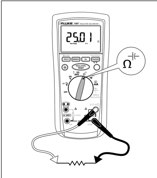
Figure 8. Measuring Resistance
