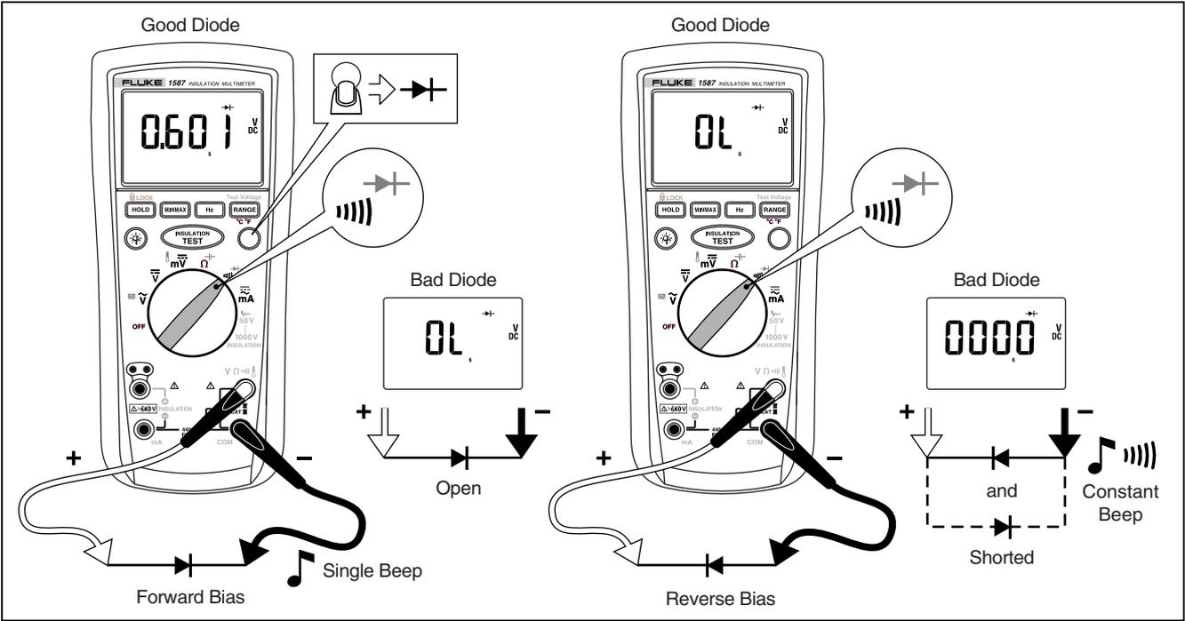
Figure 11. Testing Diodes
