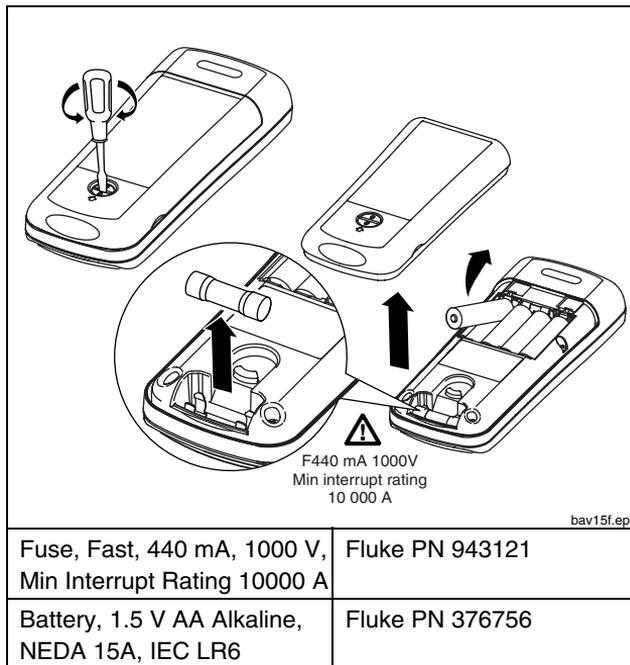
**Figure 16. Replacing the Fuse and Battery**
