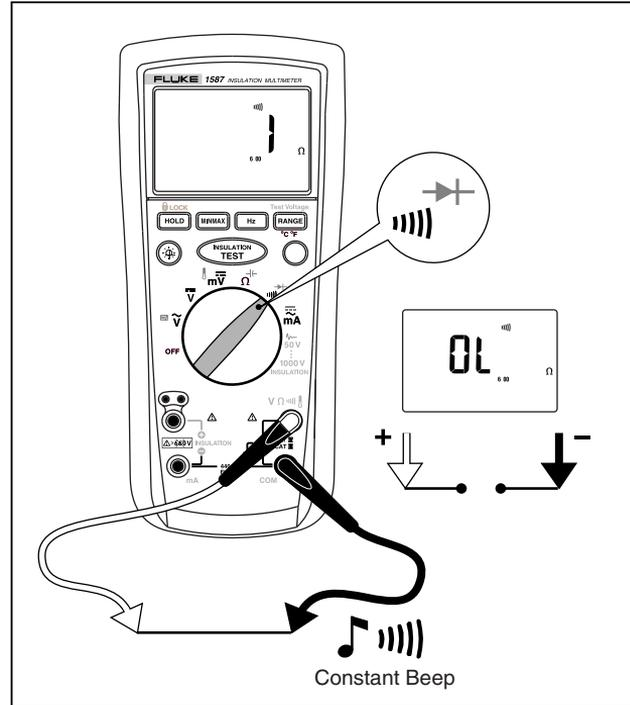
Figure 10. Testing for Continuity
